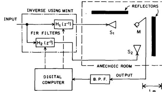
Fig. 8. Experimental conditions for inverse filtering in a sound field.  $S_1$ ,  $S_2$ : loudspeaker,  $M$ : microphone, BPF: band-pass filter intended for 315–3150 Hz. The number of taps of FIR filter  $H_i(z^{-1})$  ( $i = 1$  or  $2$ ) in the LSE method is 700, and that of  $H_i(z^{-1})$  in the proposed method is 350.
