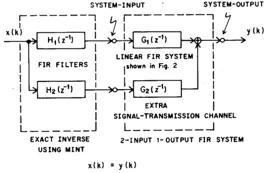
Fig. 3. Proposed inverse-filtering method based on the multiple-input/output inverse theorem (MINT).
