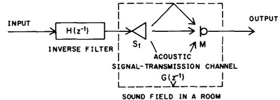
Fig. 1. Acoustic system consisting of a loudspeaker and a microphone.  $S_1$ : loudspeaker,  $M$ : microphone,  $G(z^{-1})$ : acoustic signal-transmission channel that corresponds to a room impulse response.
