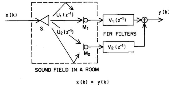
Fig. 6. Dereverberation using the proposed method.  $S$ : sound-source,  $M_1$ ,  $M_2$ : microphone,  $U_1(z^{-1})$ ,  $U_2(z^{-1})$ : acoustic signal-transmission channel.
